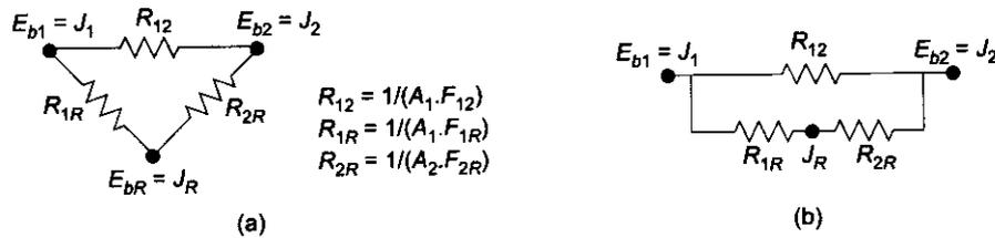
**FIGURE 13.33** Two black surfaces connected by a third re-radiating surface and its radiation network
