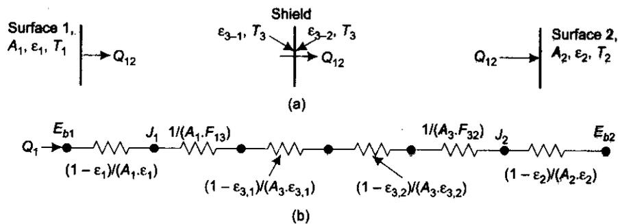
**FIGURE 13.37** Radiation shield between two parallel plates, and associated radiation network
