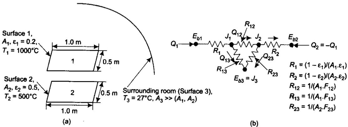
**FIGURE** Example 13.24 Two grey surfaces surrounded by a large room
