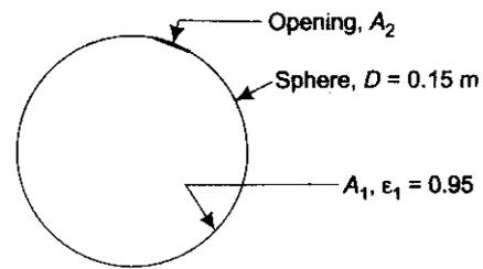
**FIGURE** Example 13.21 Hole on the surface of a sphere—hohlraum
