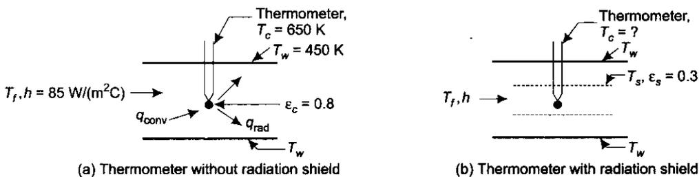
**FIGURE** Example 13.30 Radiation shielding of thermometers
