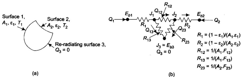
**FIGURE 13.34** Two grey surfaces surrounded by a re-radiating surface
