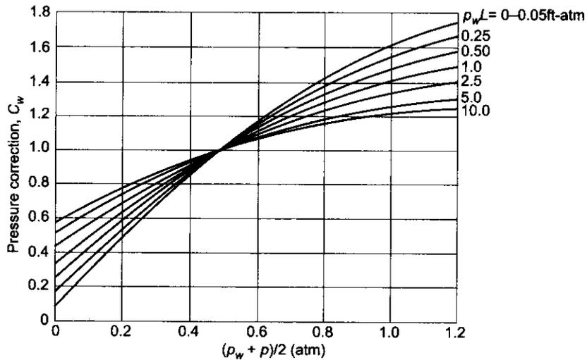
**FIGURE 13.42** Correction factor for emissivity of water vapour when the total pressure of mixture is other than 1 atm. (Source: Incropera and Dewitt [1998]. op. cit.)
