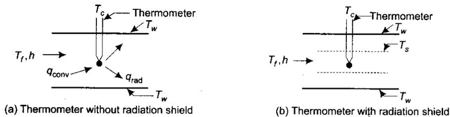
FIGURE 13.39 Radiation shielding of thermometers
