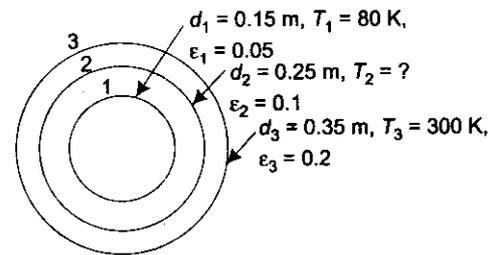
**FIGURE** Example 13.19 Three concentric cylinders
