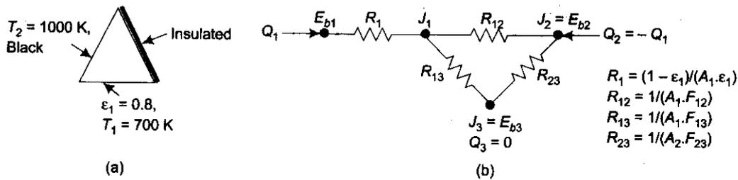
**FIGURE** Example 13.22 One black surface, one insulated surface, and one grey surface forming an enclosure, and its radiation network
