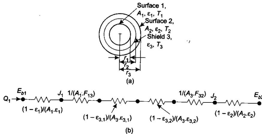
**FIGURE 13.38** Radiation shield between two concentric cylinders, and associated radiation network
