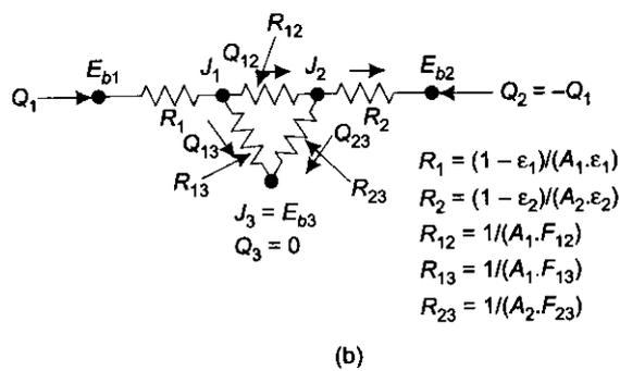
**FIGURE** Example 13.23 Two gray surfaces surrounded by a re-radiating surface
