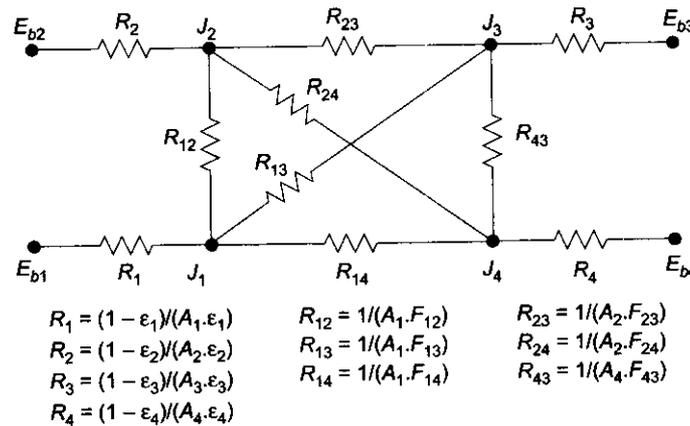
FIGURE 13.36 Radiation network for an enclosure of four grey surfaces
