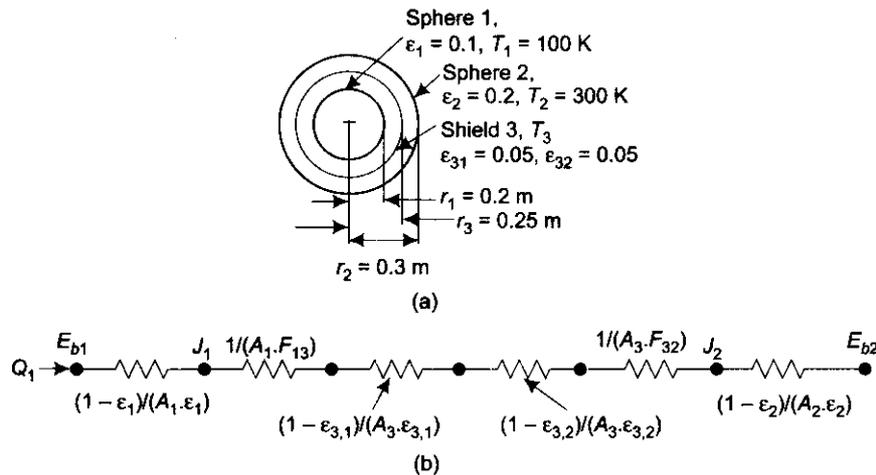
**FIGURE** Example 13.29 Radiation shield between two concentric spheres, and associated radiation network
