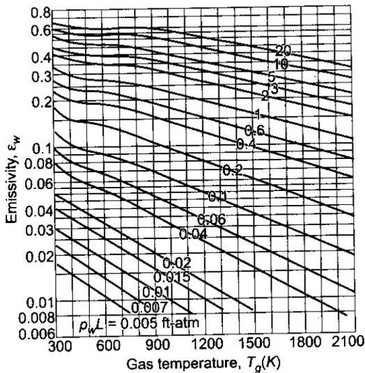
**FIGURE 13.41** Emissivity of water vapour in a mixture of other gases which are non-radiating, at a total pressure of 1 atm. (Source: Incropera, Frank P. and David P. Dewitt [1998]. *Fundamentals of Heat and Mass Transfer*. Pub.: John Wiley & Sons)
