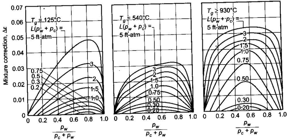
**FIGURE 13.45** Correction factor for mixtures of carbon dioxide and water vapour. (Source: Incropera and Dewitt [year]. op. cit.)
