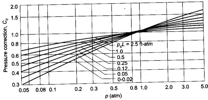
**FIGURE 13.44** Correction factor for emissivity of carbon dioxide when the total pressure of mixture is other than 1 atm. (Source: Incropera and Dewitt [1998]. op. cit.)
