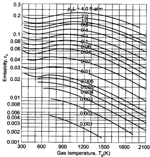
**FIGURE 13.43** Emissivity of carbon dioxide in a mixture of other gases which are non-radiating, at a total pressure of 1 atm. (Source: Incropera and Dewitt [1998]. op. cit.)
