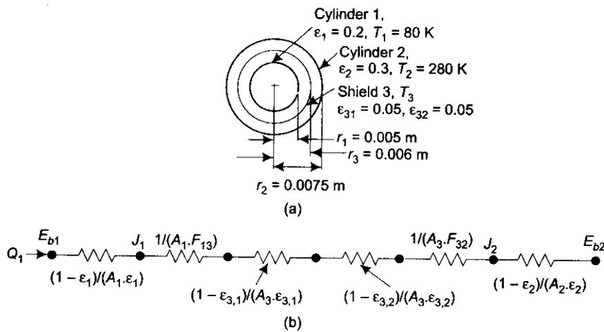
**FIGURE** Example 13.28 Radiation shield between two concentric cylinders, and associated radiation network
