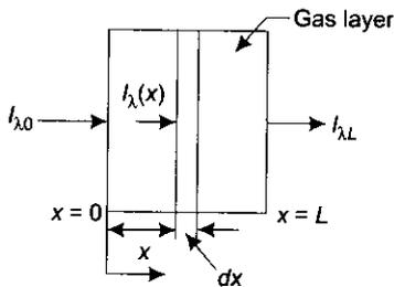
**FIGURE 13.40** Absorption of monochromatic radiation in a gas layer
