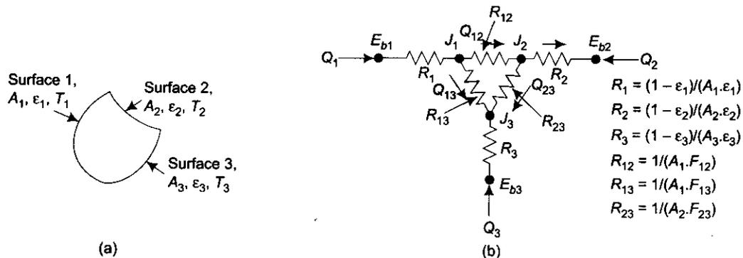
FIGURE 13.32 Three-surface enclosure and its radiation network
