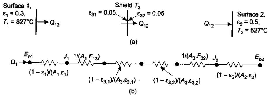
**FIGURE** Example 13.25 Radiation shield between two parallel plates, and associated radiation network
