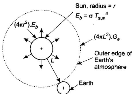
**FIGURE 13.46** Estimation of surface temperature of sun when the solar constant is known
