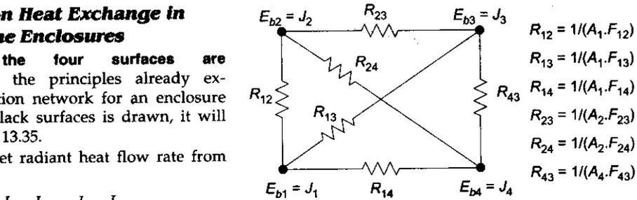
FIGURE 13.35 Radiation network for an enclosure of four black surfaces
